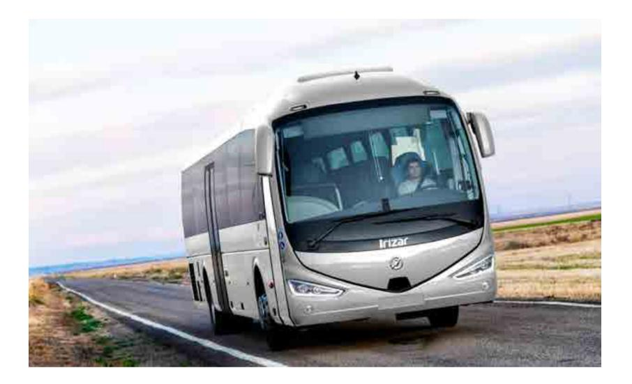
The new generation Irizar i4 coach now offers significant new features that mainly focus on a major reduction in weight and optimal per axle load distribution. The result is a **lightened** vehicle with a weight reduction of up to 955 kg, depending on the configuration chosen.
